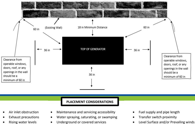
No operable windows and/or openings in the wall is permitted within 5 ft from any point of the generator
